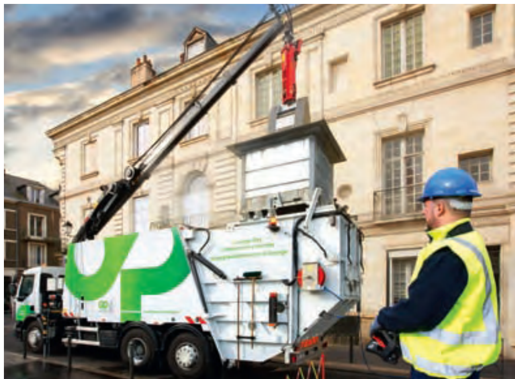
Underground, semi-underground and aboveground voluntary waste disposal containers must be kept clean. Plastic Omnium offers a multi-brand solution with a special truck that can lift and wash all types of container.
