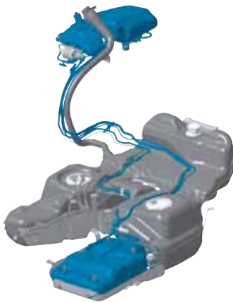
DINOx urea storage and release system for the Audi Q7.
